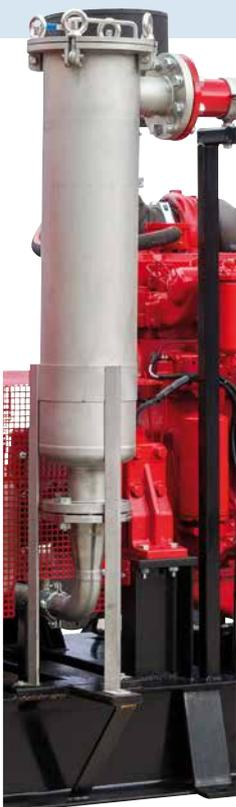
The **HI-PR Firepack** is built around the high pressure plunger pumps which are rated at 160 bar. These pumps are cooled as well as lubricated by the water itself and therefore maintenance free. Depending on the required capacity multiple pumps are driven by the same diesel engine through a gearbox.
