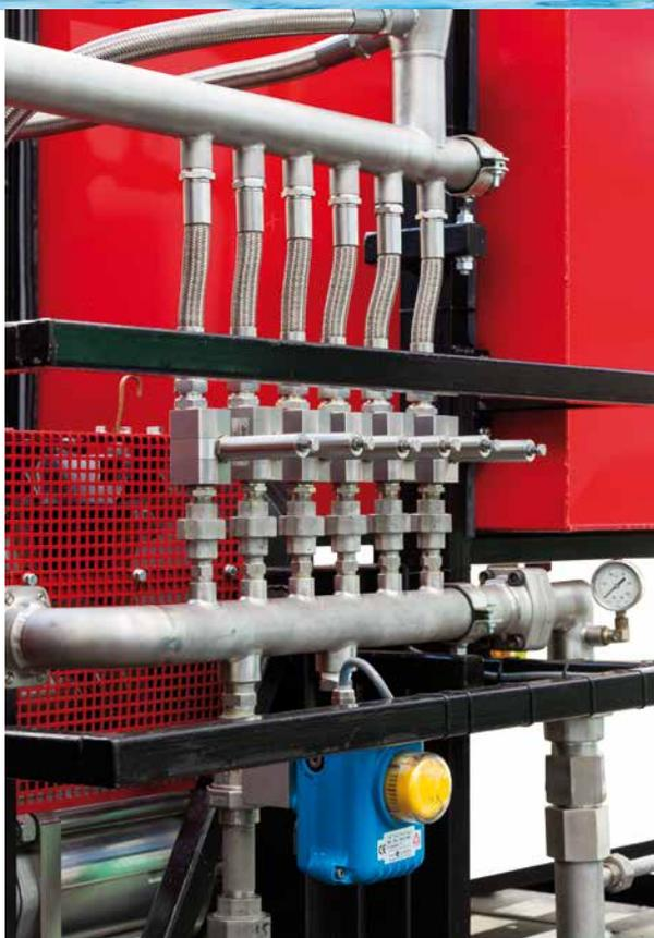
The pump pressure of the **HI-PR Firepack** is controlled by means of purpose designed control valves. These pilot controlled valves are much more stable than the usual spring loaded valves. For a diesel **HI-PR Firepack** unloading the pumps is required for starting and stopping the diesel engine. This is performed by electric controlled ball valves, which of course work with 24V from the batteries, ensuring autonomous operation.
